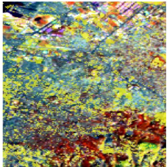
Figure 8. Result of change detection: the areas affected by fires are highlighted in yellow. Haiti, 2010
